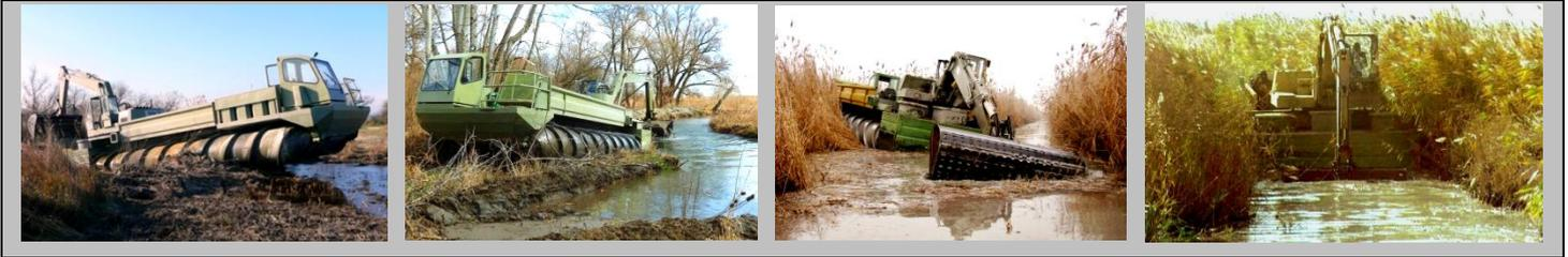
The **AMPHI-CAT** is an **amphibious vehicle** that is proven to perform in environments -- where wheel- and track vehicles would sink and ships would run aground, examples include:
